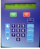
Using the up and down arrow keys scroll to the vacuum pump oil change screen.
