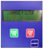
•Using the up and down arrow keys scroll through the menu options until the filter change screen is displayed –
